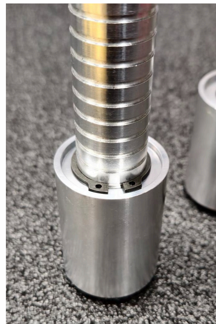
“CLIP ROD AND RETAINING RING SEATED IN SPRING SPACER
