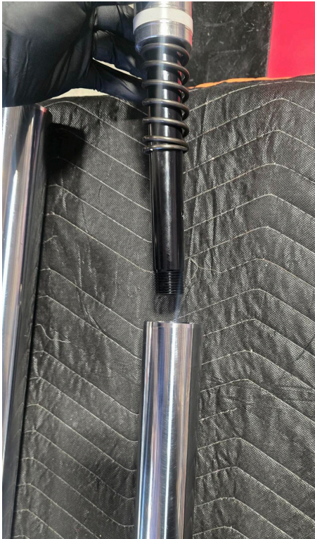
DAMPNER ROD WITH TOPOUT SPRING GOING INTO UPPER FORK TUBE
