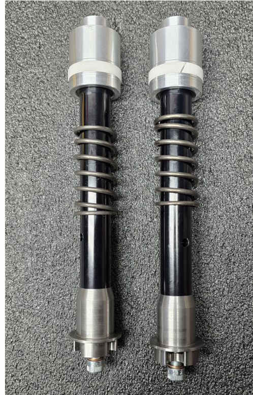
AMERICAN SUSPENSION VALVED DAMPNER RODS
