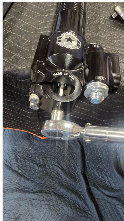
FORK DRAIN BOLT TORQUE TO 18 FT. LB
