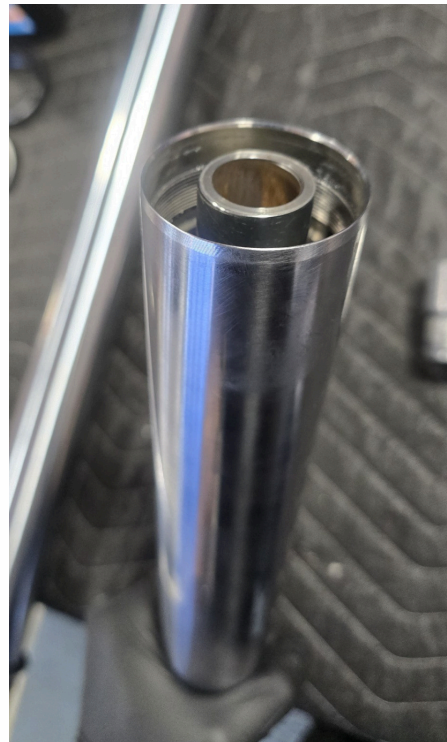
CLIP ROD SPACER (UPDATED FK KITS ARE THREADED ONTO THE CAP) DEPICTED SITTING 1/2 " ABOVE THE FORK TUBE THREADS
