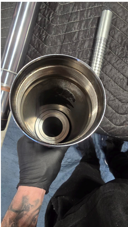
HOW SPRING SPACER SHOULD LOOK ONCE INSTALLED
