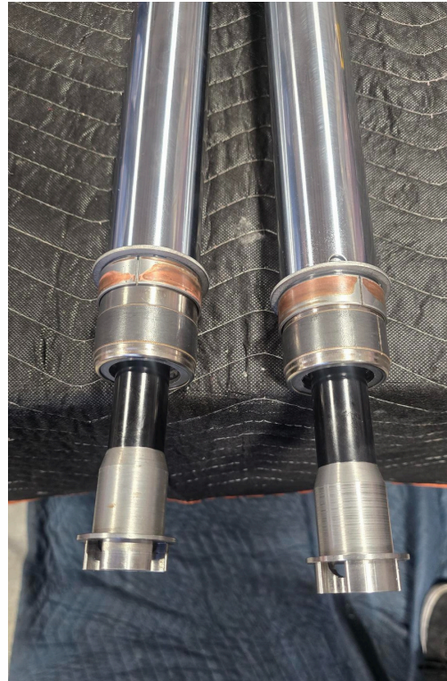
DAMPNER RODS INSTALLED WITH FORK TUBE BUSHINGS IN PROPER ORIENTATIO N AND DAMPNER ROD SEAT INSTALLED
