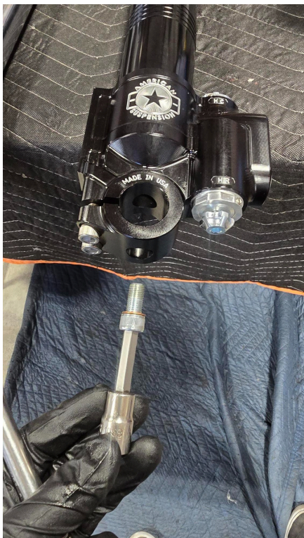
FORK DRAIN BOLT AND COPPER CRUSH WASHER INSTALL
